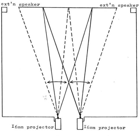
During projection each projector is moved into one or all three of the above co-ordinate screen shapes.
